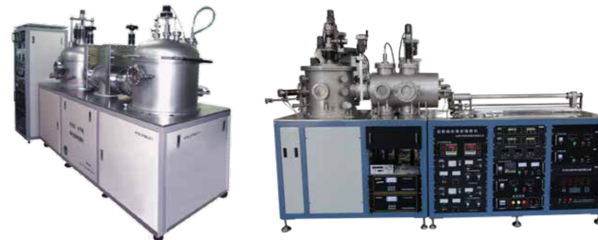
热蒸发、电子枪、多弧、磁控溅射等多功能镀膜机 Multi-functional Coating Machine of Thermal evaporation, Electron gun, Multi arc, Magnetron sputtering, etc
