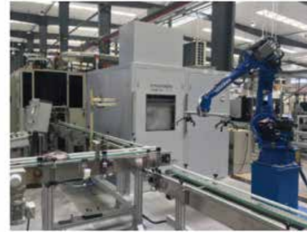
真空氦检漏设备 Vacuum helium leak detection equipment
